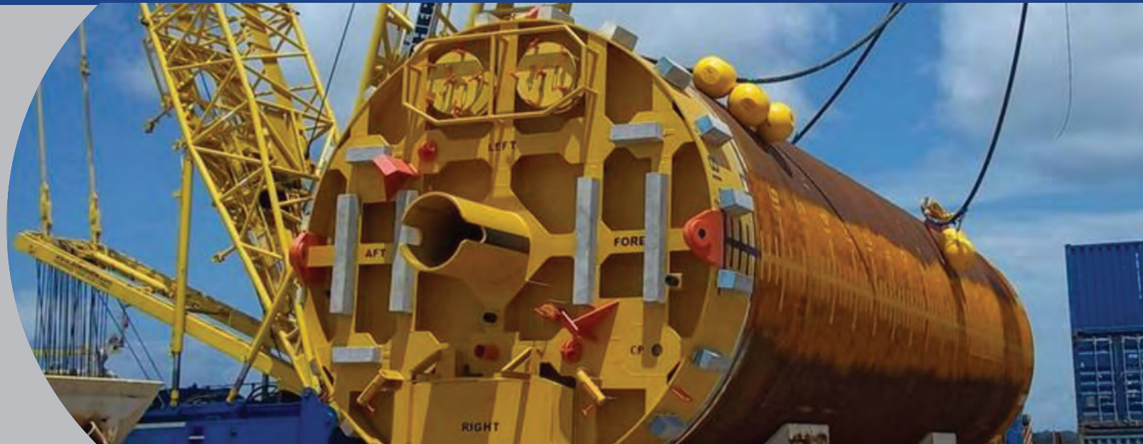
Vent caps installed on top of suction pile of a major E&P company
